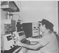
Lab Asiantante Alberio Petrochi analyzes the lead content of a gasoline at the Labs new electronic Atomic Absorption Spectrophotometer.
